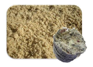
**Reusable product** with a **high calorific value** (up to 7000 kcal / kg) and therefore can be classified as **RDF** (European Waste Catalogue **Code: 19 12 10**).
